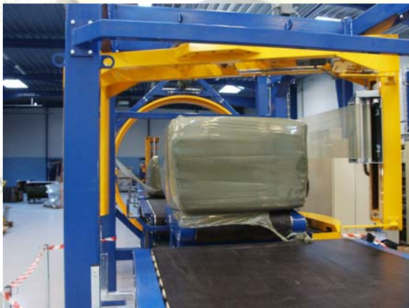
STEP 1: Horizontal packaging in the W3000 swing arm wrapper.
