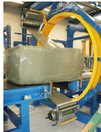
STEP 2: Vertical packaging in the vertical ring machine.
